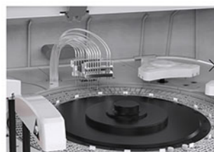
Reaction Tray 37±0.1°C, water bath.
