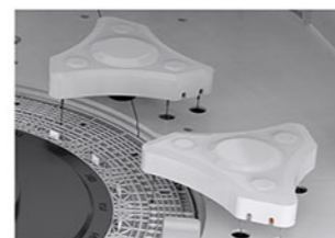
Mixer Probe Dual mixer, auto frequency adjustment.
